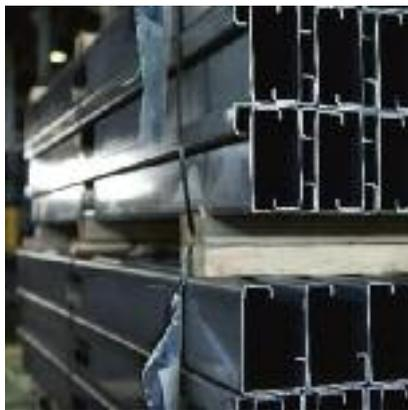
in general, is predominantly galvanized steel, typically high-strength, low-alloy material. The company's roll formers can effectively handle 26-gauge material up to  $\frac{3}{8}$ -inch material.
